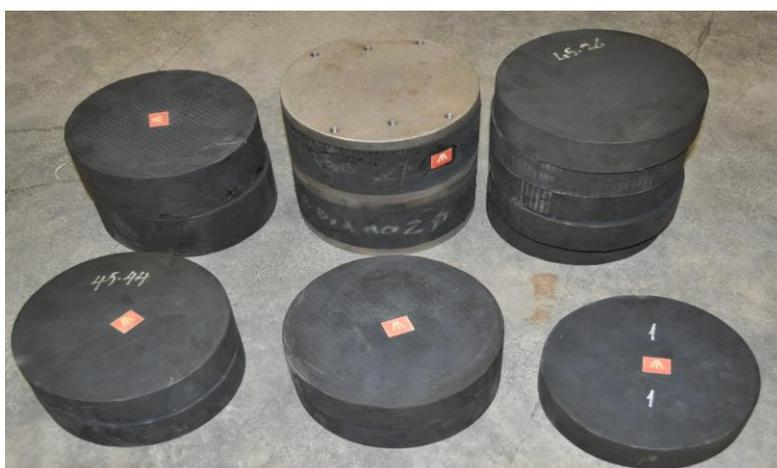
Figure 29: FREIs used at the testing campaign
