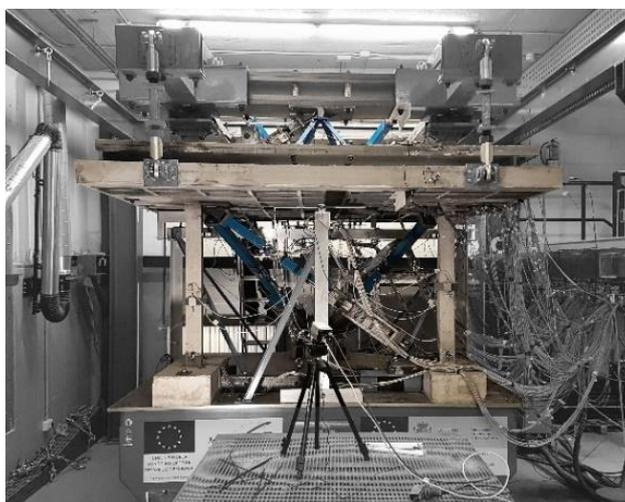
Figure 19: General overview of the test specimen installed in the shake table
