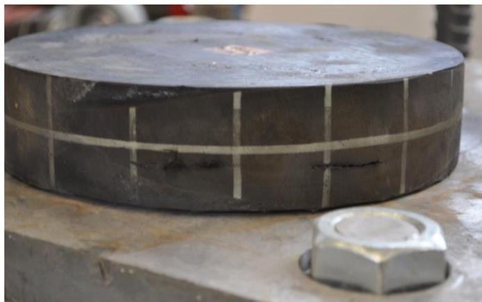
Figure 49: Ruptures in bearing observed after test frb08
