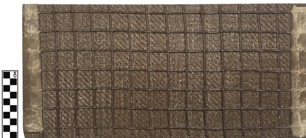
Figure 91. PowerRibs composite plate (420x200x2 mm) produced by Bcomp.
