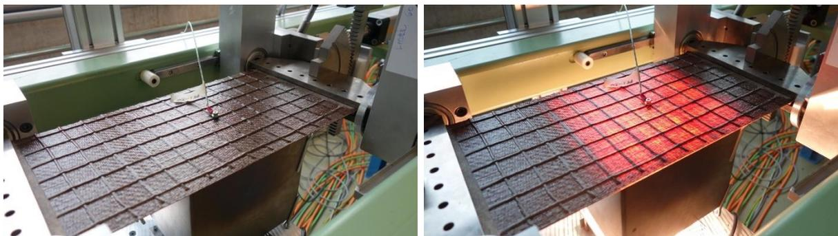
Figure 93. Tested composite plate specimen with inactive (left) and active (right) IR lamp
