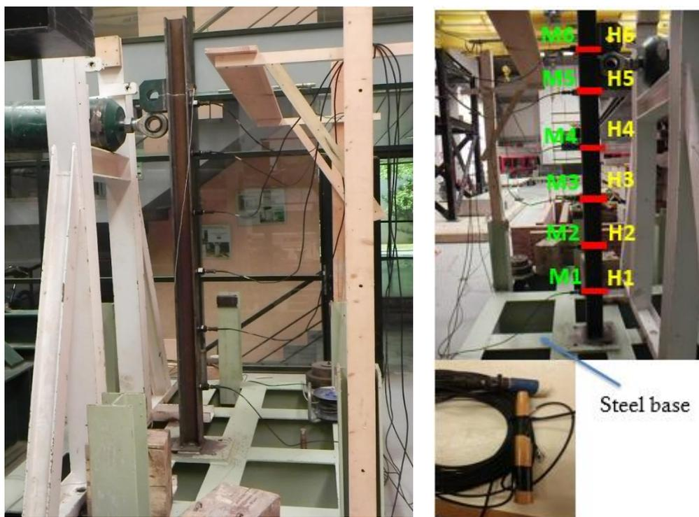
Figure 75: Column hammer test
