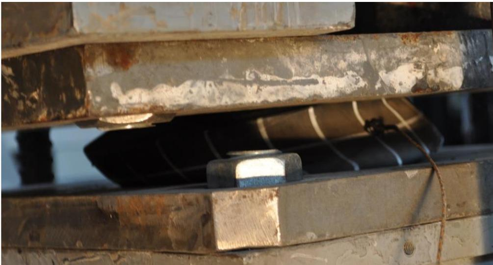
Figure 38: Photo of the top bearing in phase 1 (roll-out effect)
