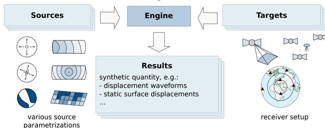
**Figure 2.** The architecture of the *Pyrocko-GF* and object oriented implementation. The *fomosto* program is a command-line interface (CLI) to create GFs using the backends, to inspect and manage *GF stores*. b) The *engine* is the central object that accesses the computed *GF stores* and calculates the synthetic waveforms based on the specified source (e.g. moment tensor, double-couple source or finite-
