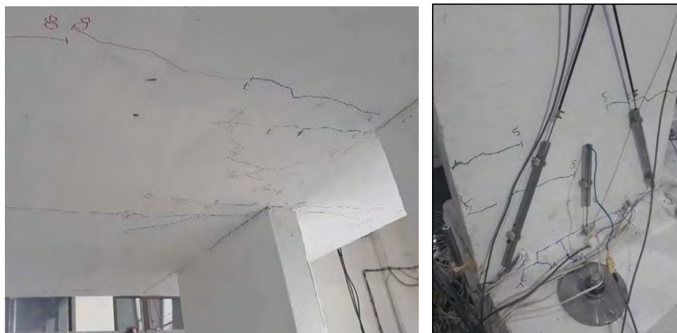
Figure 356: Cracks in second slab(left) and pier foundation contact (right)
