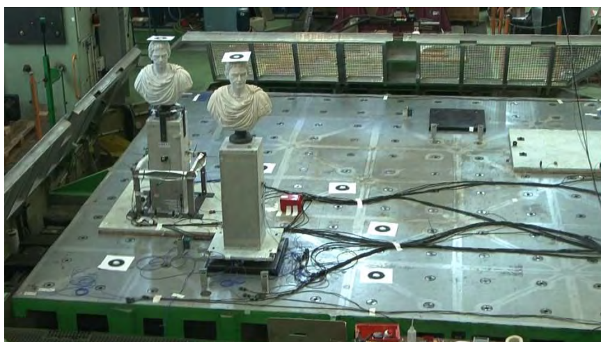
Figure 120: Configuration I-3: Augusto bust on hollow pedestal; on marble and on SMA isolator
