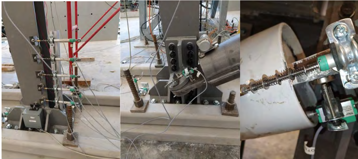
Figure 234: Some details on the instrumentation for the 2D test: Column potentiometers and column base inclinometer (left), elastic brace connection potentiometer to measure relative displacement (centre) BRB potentiometer to measure BRB deformation (right)
