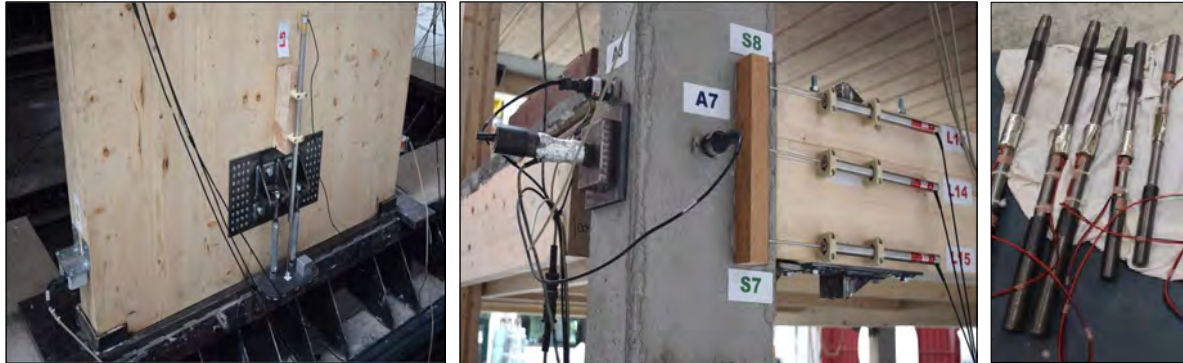
Figure 156: Monitoring system – LVDTs/potentiometers at the base of a timber wall (left), load-cell, accelerometers and LVDTs monitoring a beam-column joint (centre), “Plug&Play” dissipaters (right)
