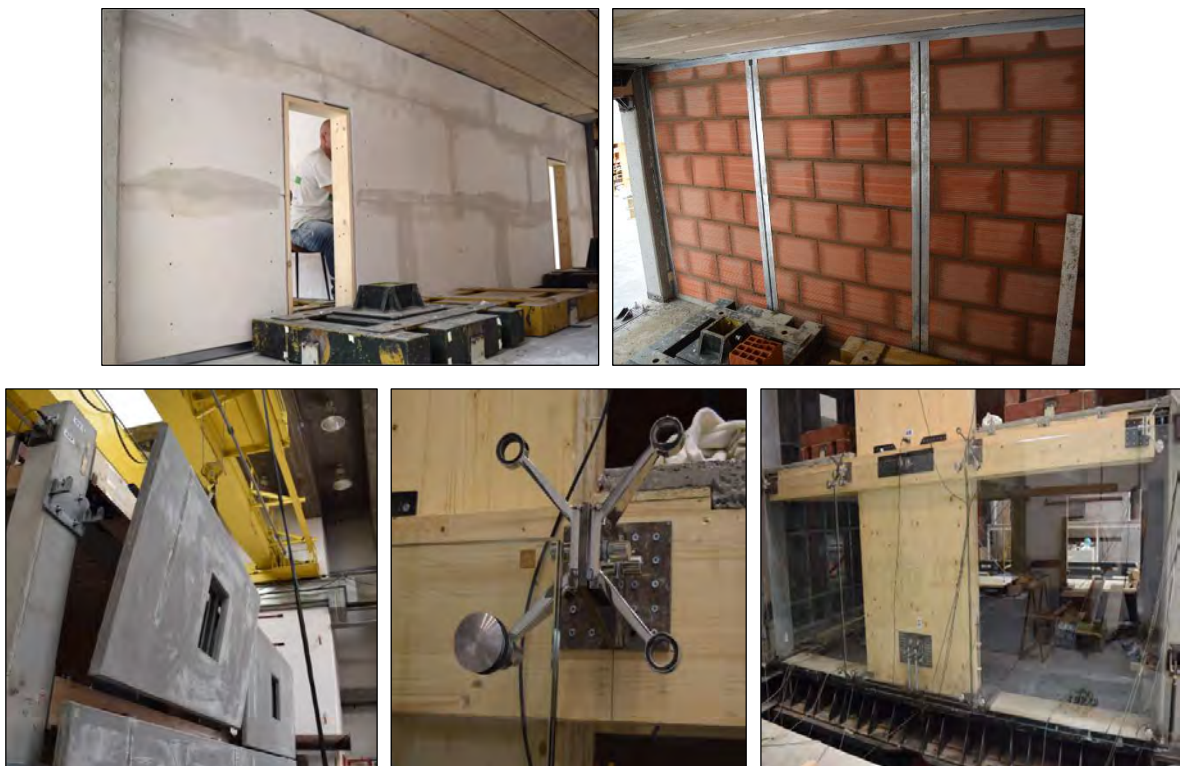
Figure 153: Non-structural elements – fiber-reinforced gypsum partition (top, left), low-damage masonry infill wall (top, right), GFRC façade system in the frame direction (bottom, left), detail of the hinge spider-plate assembly (bottom, centre), assembly of the spider glazing façade in the wall direction (bottom, right)
