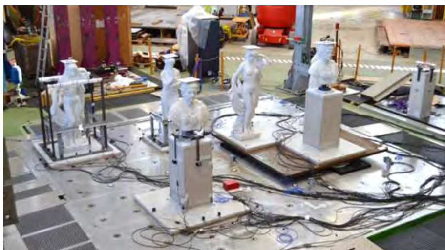
Figure 123: Configuration II: Non-isolated vs isolated statues (friction pendulum system). The pairs of specimens compared are: (i) Traiano bust on solid pedestal, (ii) Fanciulla and (iii) Figura femminile
