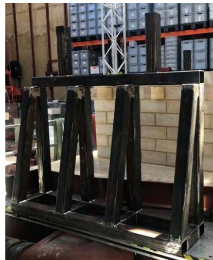
Figure 274: Support system design with celsius SHS 100x100 steel frame
