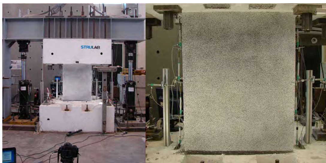
Figure 209: DIC system and speckle pattern
