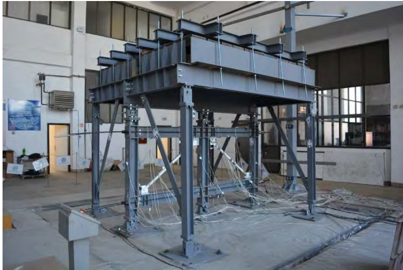
Figure 376: Testing model assembled on IZIS shake table
