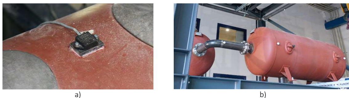
Figure 90: Instrumentation of tanks and pipes on the 2 nd floor: a) Accelerometer on top of the horizontal tank, b) Markers on horizontal tanks and pipes
