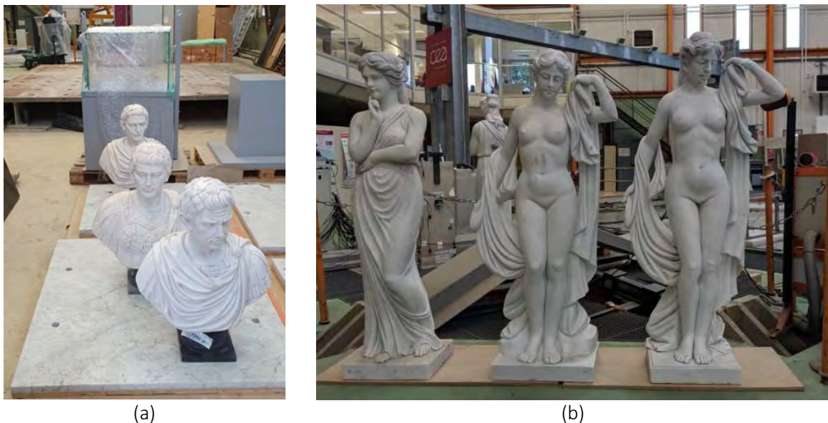
Figure 113. Components used for the shake table tests: (a) Busts and display case, (b) female statues
