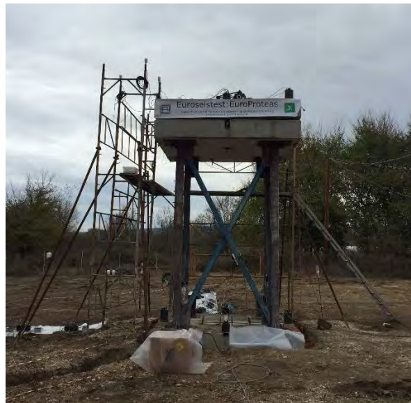
Figure 463: A 2D sketch and a view of EUROPROTEAS prototype structure
