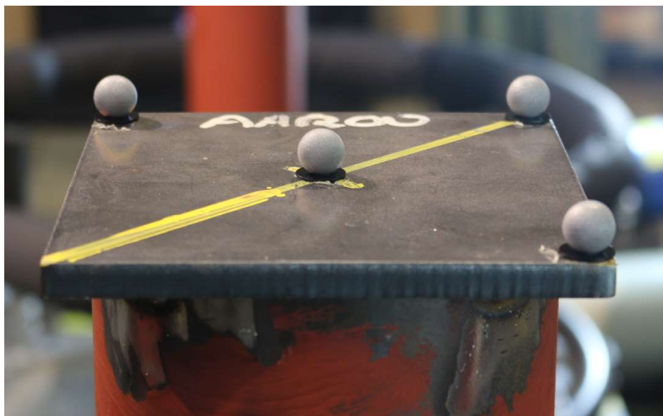
Figure 261: Markers on top of a free rocking column
