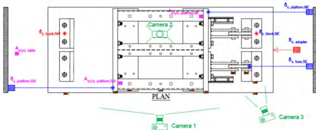
Figure 294: The modified instrumentation plan that was used during testing
