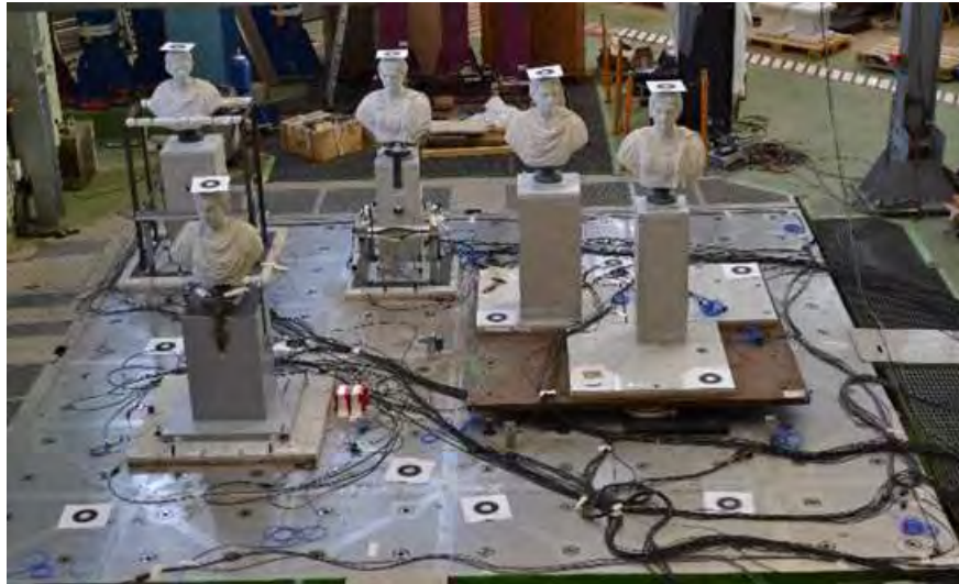
Figure 124: Configuration III: Non-isolated vs isolated statues (friction pendulum system). The pairs of specimens compared are: (i) Tito bust on metallic pedestal, (ii) Augusto bust on solid pedestal, and (iii) Traiano bust on hollow pedestal
