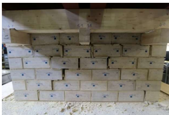
Figure 284: Diagonal failure of specimen A at GM level A9 (140% - only H)
