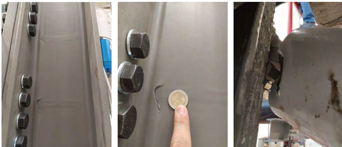
Figure 236: Damage observed on the retrofitted frame during the pseudo-dynamic test
