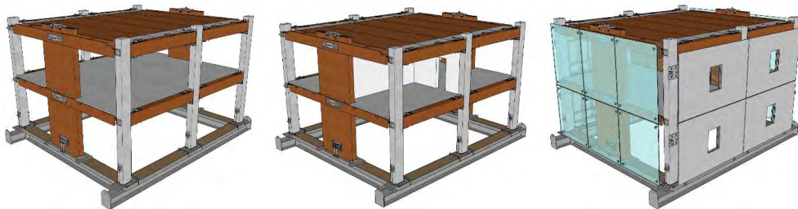
Figure 150: Test specimen configurations – Skeleton Building (left), Option1 (centre), Option2 (right) (Pampanin et al., 2020)
