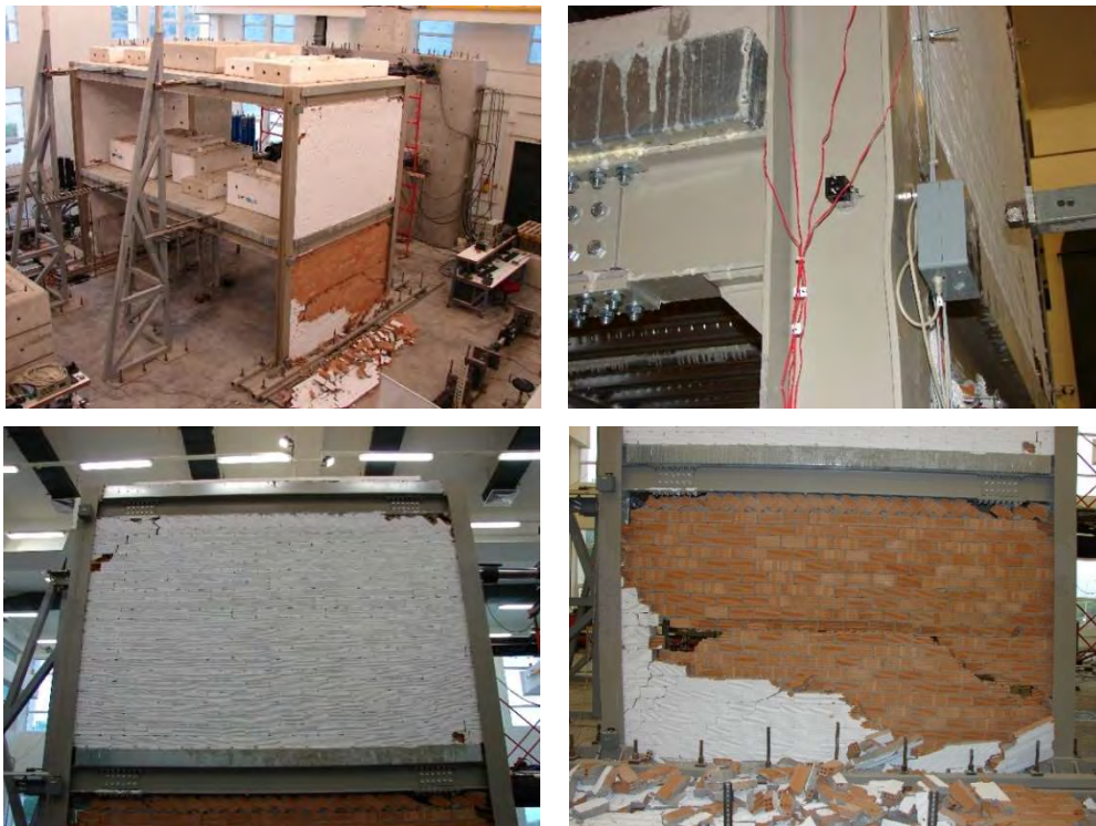
Figure 235: Damage observed on the infilled frame during the pseudo-dynamic test
