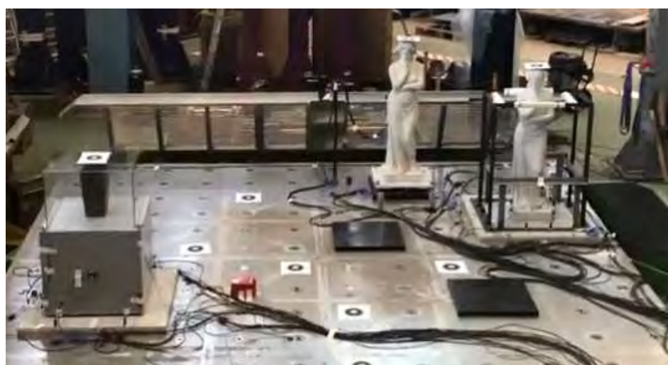
Figure 122: Configuration I-5: Female statue (Fanciulla) standing on the ground pedestal and non-isolated display case and non-isolated display case
