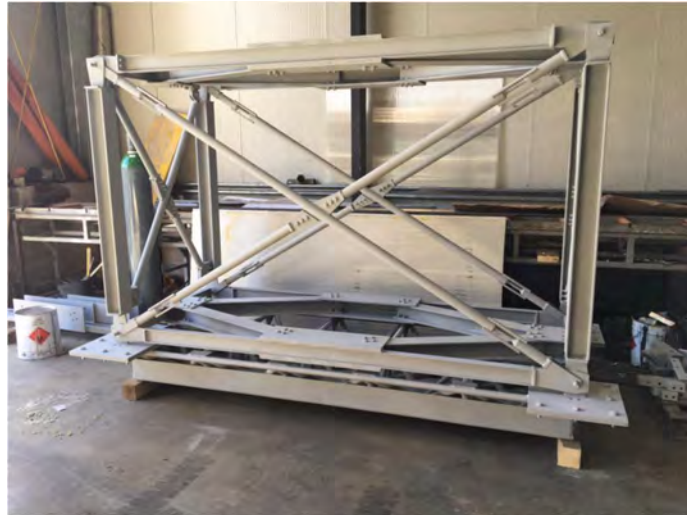
Figure 344: The manufactured and assembled CBF to be tested
