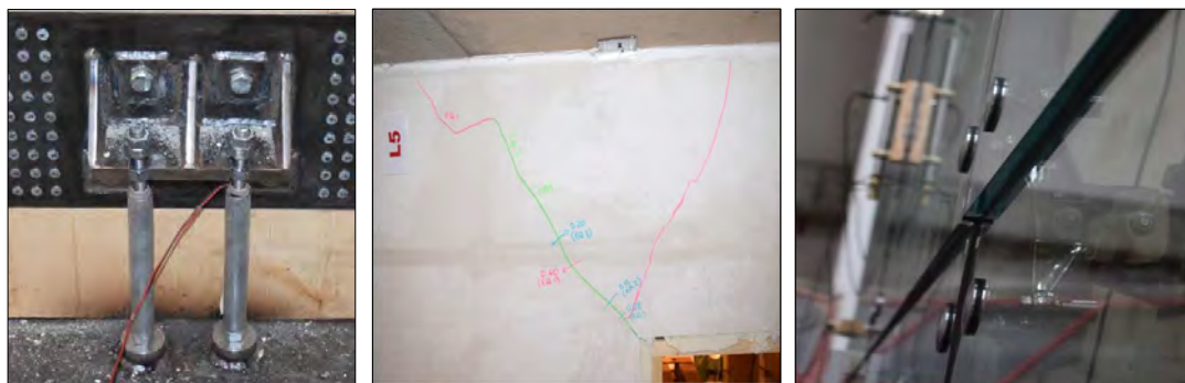
Figure 158: Yielding of the external wall dissipaters (left), diagonal cracking of the gypsum partitions (centre), out-of-plane displacements of the glass panels (right)
