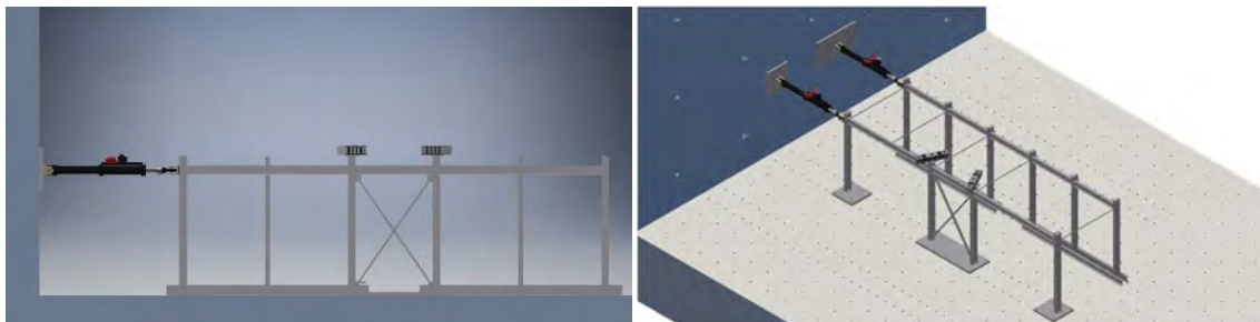
Figure 9: Side view (left) and bird's-eye view (right) of the specimen and set up at the ELSA Reaction Wall
