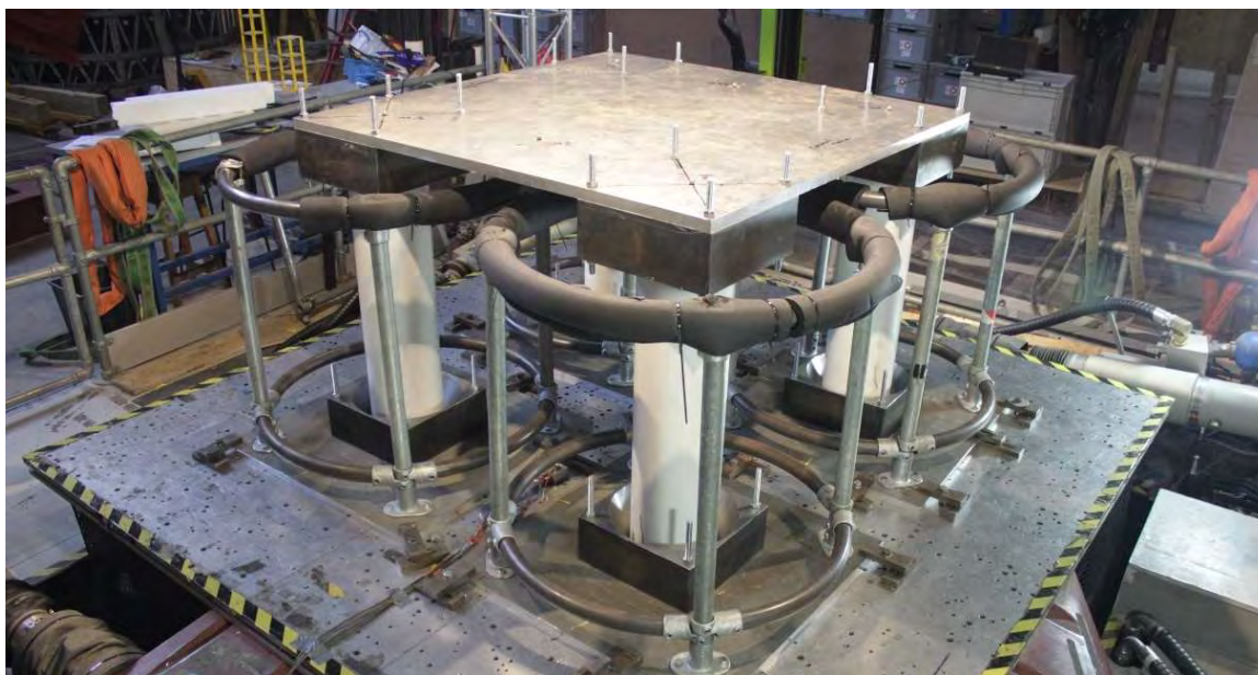
Figure 258: Wobbling Frame specimen on the University of Bristol Shake Table
