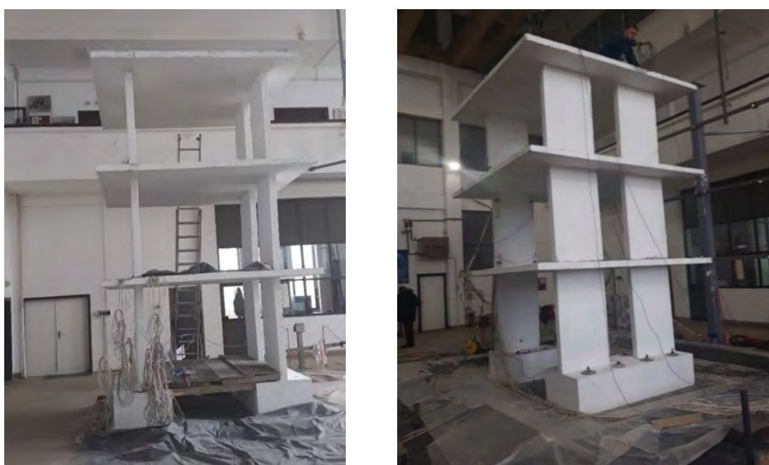
Figure 347: Laboratory specimen after construction (left) and mounted on the shaking table (right)
