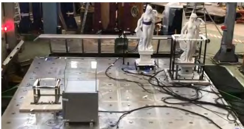
Figure 121: Configuration I-4: Female statue (Figura femminile) standing on the ground pedestal and non-isolated display case and isolated display case (SMA isolator)
