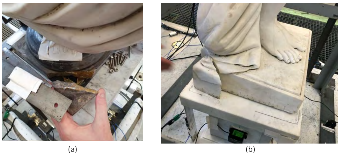
Figure 133. Typical damage at the base of the specimens: (a) bust, (b) base of the statue
