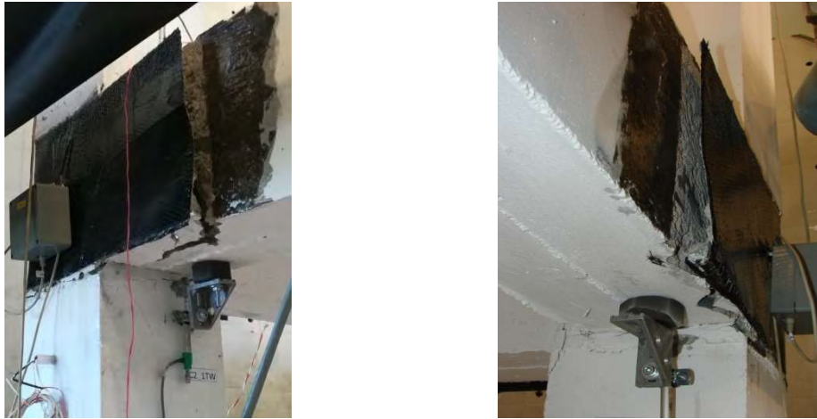
Figure 199: Detachment of anchorage of FRP overlay of joints from lateral face of beam, through the concrete substrate
