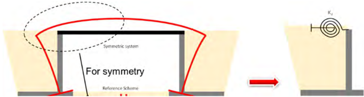
Figure 241: Assumption made for determining the thickness of the bridge deck
