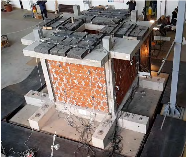
Figure 395: Completely instrumented and loaded test specimen placed on shake table
