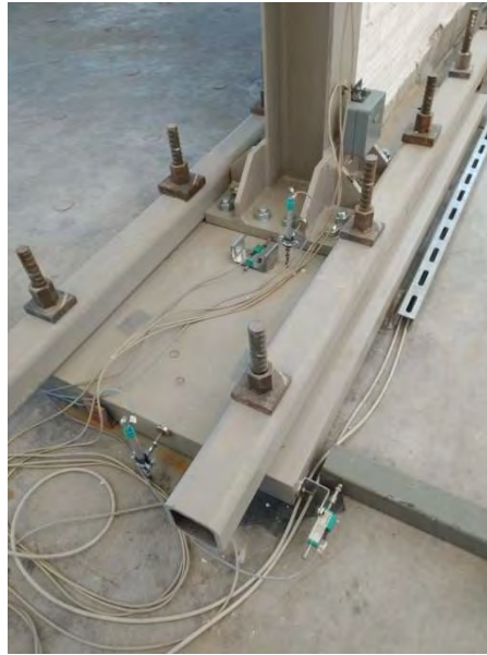
Figure 230: Typical configuration of the structures' foundation.
