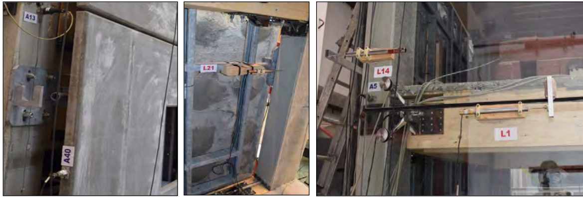
Figure 157: Monitoring system – sensors on the fiber-reinforced gypsum partition in the frame direction (top, left); LVDT transducers on a lateral low-damage masonry wall and accelerometer at the middle of the panel (top, centre and right); accelerometer at the middle of the GFRG panel (bottom, left) and LVDT monitoring the anchorage-column relative displacement (bottom, centre); transducers recording the glass/column and glass/glass displacements (bottom, right)
