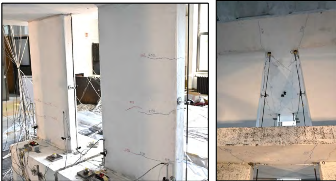
Figure 371: Cracks in walls (left) and slabs (right)
