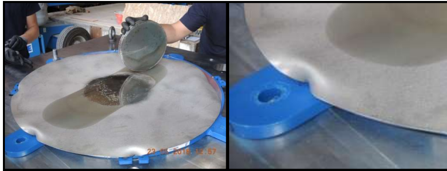
Figure 32: Test of VSP and failure of the high friction sliding surface
