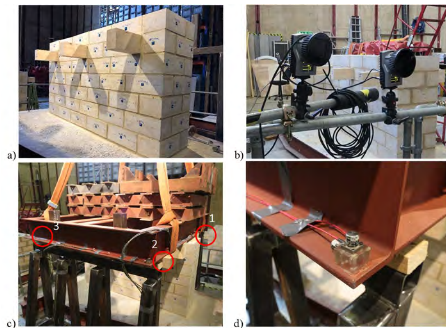
Figure 278: Control system: a) displacement markers on the stone faces to measure the displacement of each point with b) five infrared cameras; c) accelerometers on the steel frame top in three different positions; d) accelerometer detail
