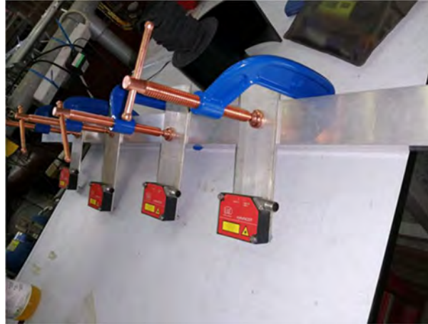
Figure 328: Non-contact displacement transducers (INDIKON type)
