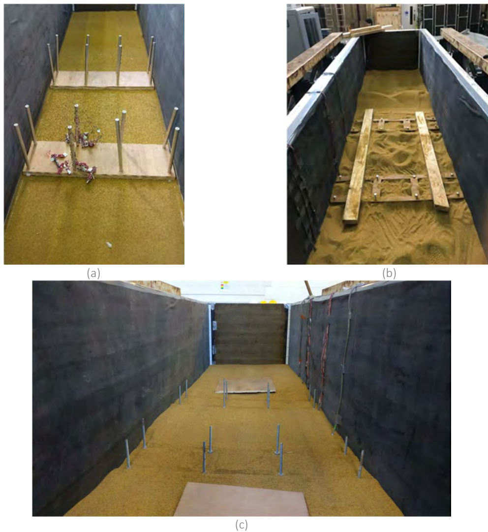
Figure 249: Actual set-up of the sand infill and bridge model (a) Piles in position inserted in the plywood plug and sitting on PU foam; (b) First sand infill and shaking (c) Second sand infill and shaking, studs in position
