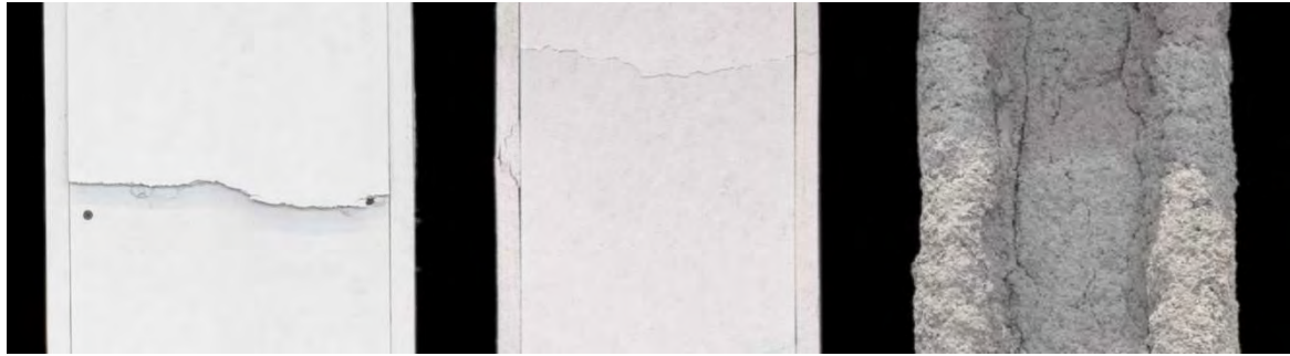
Figure 16: Damage of the fire protection elements due to the combination of seismic and fire actions: test#2 column B (left), test#3 column C (centre), test#4 column D (right)
