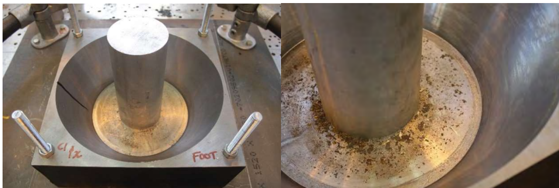
Figure 260: Left: Conical restraint with peg designed to prevent overturn in case of excessive tilt. Right: Shavings, showing that the steel column scratched the restrainer as it was "climbing out"
