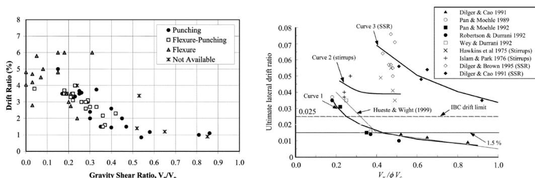
Figure 13: Ultimate drift capacity and gravity shear ratio. Test results for interior connections without transverse reinforcement (left) (Huete MB, Bai JW, 2007) and test results without and with transverse reinforcement (ACI-ASCE Committee 421, 2015) (right)
