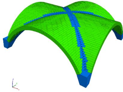
Figure 9: Masonry cross vaults numerical modeling
