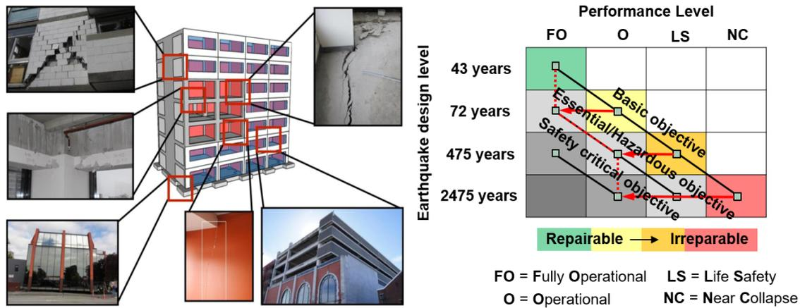
Figure 14: Left – typical damage occurring in modern RC buildings (Johnston et al., 2014); Right – seismic performance design objective matrix of SEAOC Vision 2000 (1995) modified to achieve a damage-control design philosophy (Pampanin, 2012, 2015)
