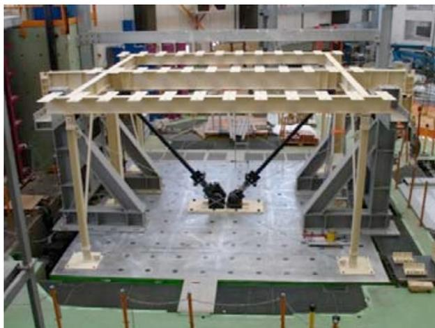
Figure 21: Test frame on Azalee shake table (CEA Saclay) without added masses showing pair of brace-gusset plate specimens (Goggins J. et al., 2018)
