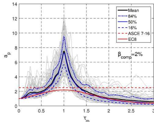
Figure 19: Mean and 16, 50, 84% percentiles for  $a_p$  as evaluated for records tuned to the fundamental period of the supporting buildings and a component damping level,  $\beta_{\text{comp}} = 2\%$ . Also shown are the  $a_p$
