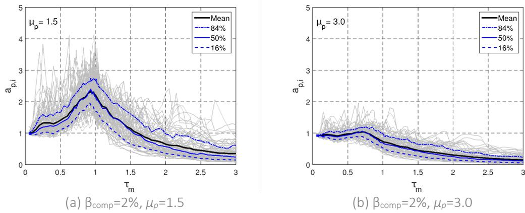
Figure 20: Inelastic floor spectra for a component damping ratio,  $\beta_{comp}=2\%$ , and two component ductility levels,  $\mu_p$  (adapted from Kazantzi et al, 2020a)
