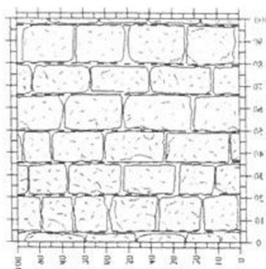
Figure 16: Aquilano apparatus for external leaves, by S. Brusaporci (2007)
