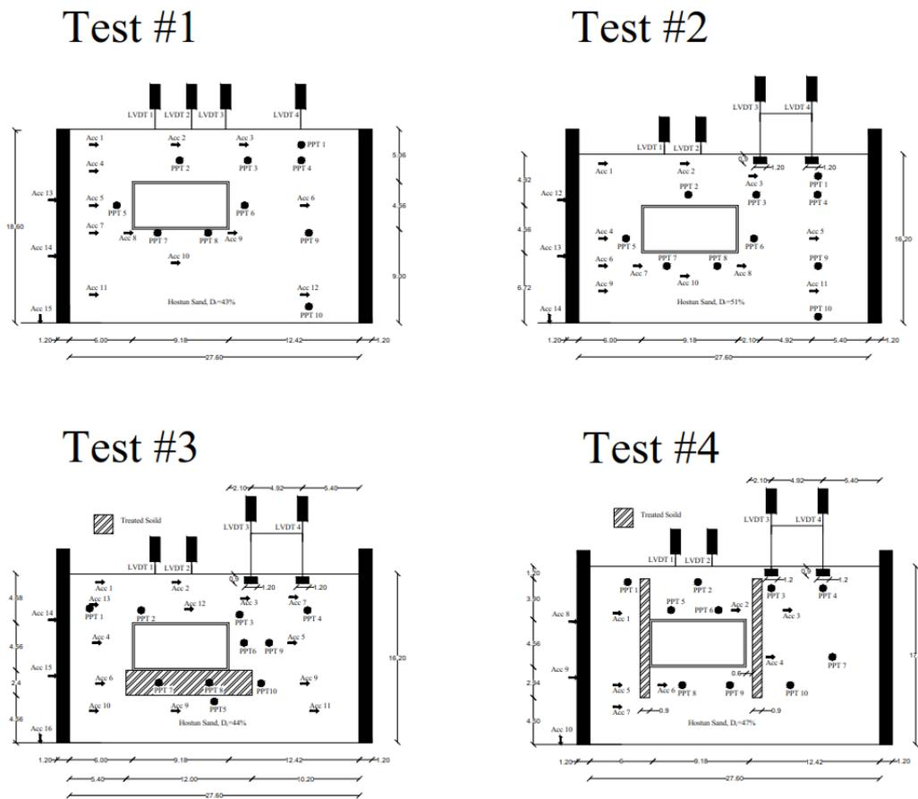
Figure 17: Schematic drawings of the four centrifuge models
