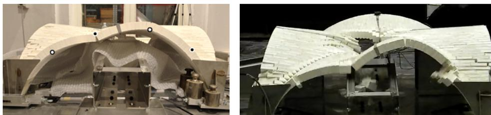
Figure 8: Masonry cross vaults shaking table tests
