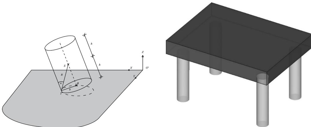
Figure 15: Left: Free rocking cylinder. Right: Wobbling frame
