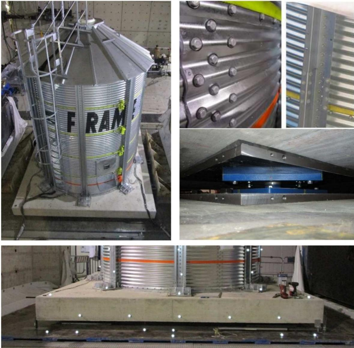
Figure 7: Full-scale grain steel silo tested both in fix base and seismic isolated configuration on the shaking table
