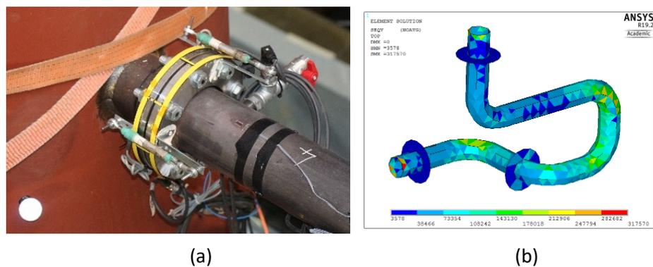
Figure 12: (a) Traditional (potentiometers, strain gages) and innovative (optic fibers, optical markers) instrumentation applied to a tank-piping-flange system; (b) 3D numerical modeling of a piping trunk
