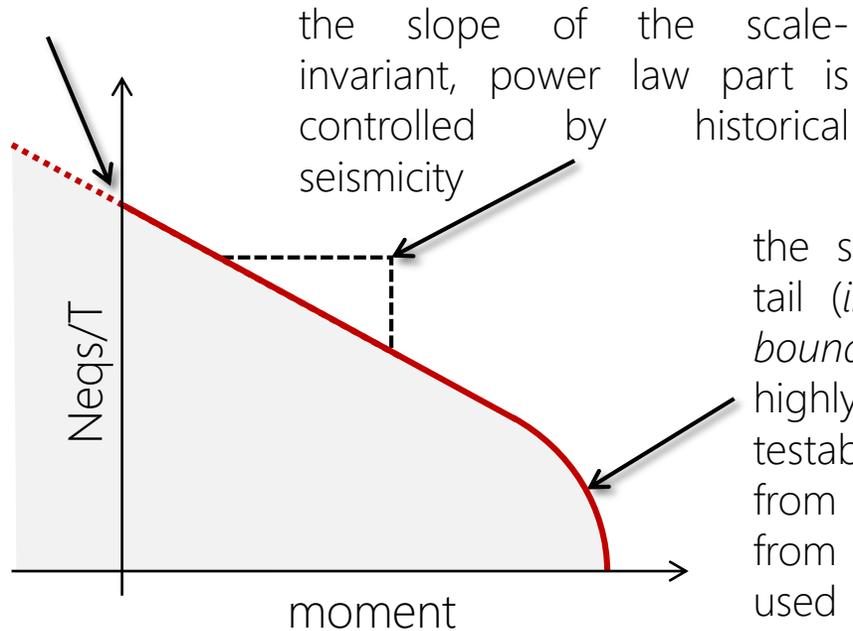
$$\begin{aligned} \chi &= 1 \\ \mu &= 30 \text{ GPa} \\ M_0 &= 1.27\text{E}+9 \text{ Nm} \leftrightarrow m_0 = 0.0 \\ M_{xp} &\leftrightarrow m_{xp} = \text{from scaling laws} \\ &\quad \text{[Leonard 2014, BSSA]} \\ \beta &= 2/3 \leftrightarrow b = 1 \end{aligned}$$
