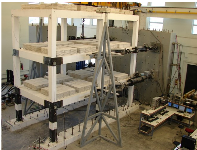
FRP retrofitted frame
