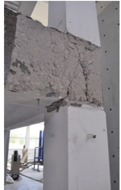
Cracking at column-foundation and column-joint interfaces of the first floor
