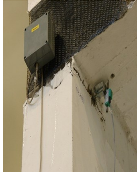
Cracking at column-foundation and column-joint interfaces of the first floor
