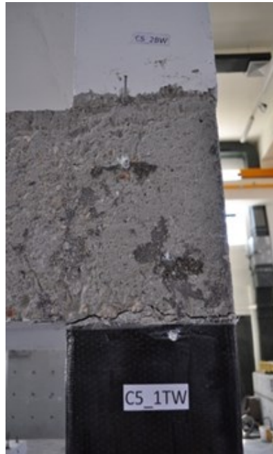
Cracking at interfaces and joints after final monotonic test
