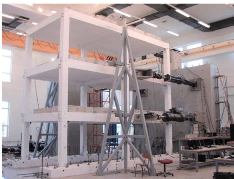
Three-story, nearly full-scale specimen in STRULAB TA facility (arrows indicate columns with continuous reinforcement – in all others, bars are spliced)
