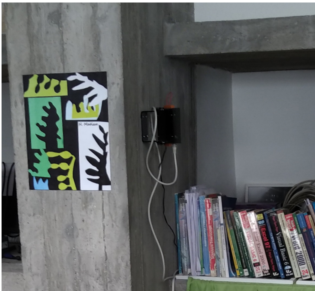
Figure 4. On October 2018, a P-Alert low cost strong motion acceleration sensor was deployed at Arsakeia schools. It was used locally and linked to NOA monitoring center in Athens via EW plugin and seedlink.
