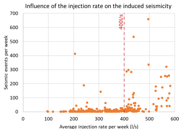
Figure 23: Influence of the injection rate on the induced seismicity from September 2011 to June 2018 (Seismic catalog SIL Network)
