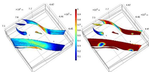
**Figure 1:** Evolution of SCU (shear capacity utilisation) at the onset (left) and after 30 years (right) of geothermal production. SCU is a measure of fault stability; faults are reactivated at SCU=1.
