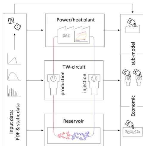
**Figure 1:** Model overview of the integrated geothermal energy model
