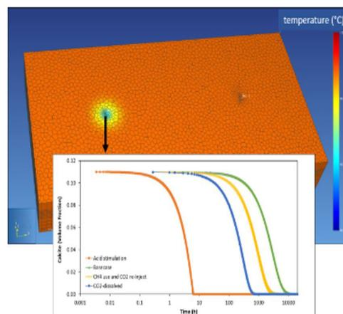
**Figure 2:** Coupled thermo-hydro-chemical models were used to model the dissolution of calcites and evolution of porosity during acid stimulations.
