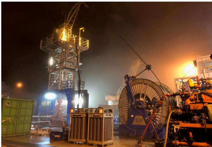
**Figure 2:** Deployment of coiled tubing in the well at the Soultz-sous-Forêts site (source: ÉS-Géothermie)
