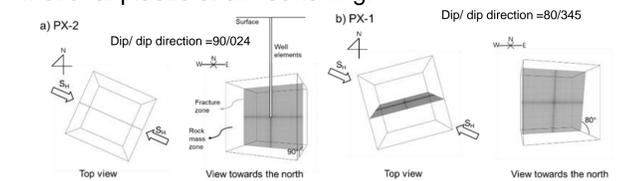
Figure 5. Model configuration of (a) PX-2 and (b) PX-1; top view and view towards the north (Yoo et al., 2021).
