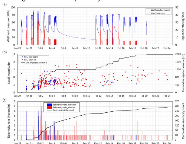
Figure 1. Overall data of the first stimulation conducted in PX-2 (Park et al., 2020).
