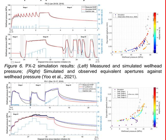
Figure 6. PX-2 simulation results: (Left) Measured and simulated wellhead pressure; (Right) Simulated and observed equivalent apertures against wellhead pressure (Yoo et al., 2021).
