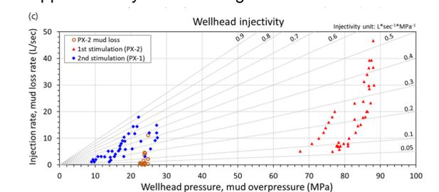
Figure 3. Wellhead injectivity during the first and second hydraulic stimulations (Park et al., 2020).
