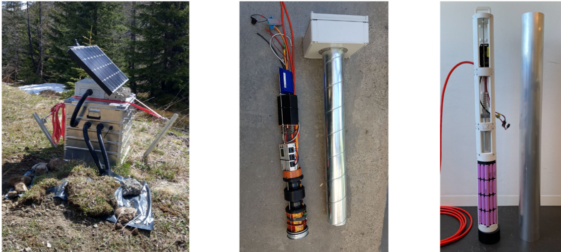
Figure 6.4.1 Prototype development stages. Left: classical mobile station from the SED aftershock pool (reference), Center: Prototype-1 built from off-the-shelf components, Right: Prototype-2 with custom casing (caps not shown), internal frame, battery, sensor and power electronics.
