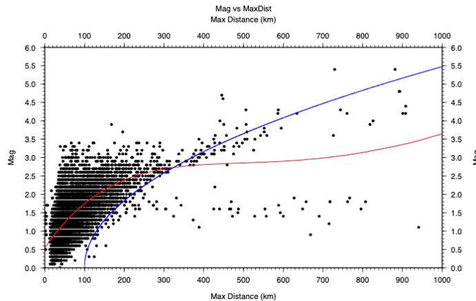
Figure 4 - Magnitude as function of distance. Red line is the not selected polynomial best fit, while the blue line is the empirical relation we used.
