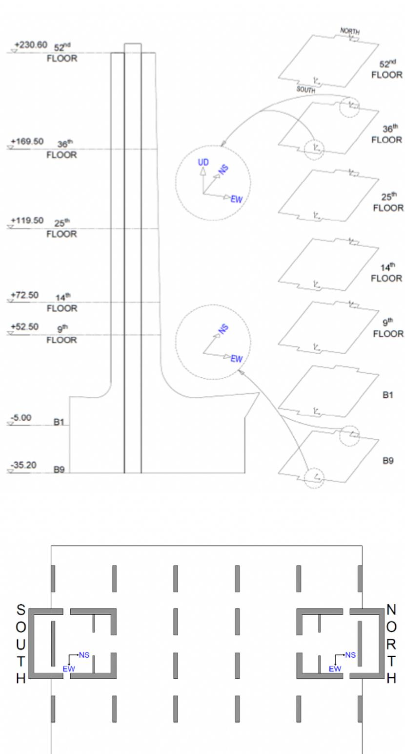
**Fig. I.4** Location and orientations of the sensors in the Sapphire building (vertical elevation and plan view).
