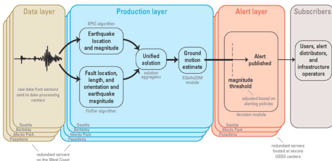
Figure II.3. From Revised Technical Implementation Plan for the ShakeAlert System (Open-File Report 2018-1155)
