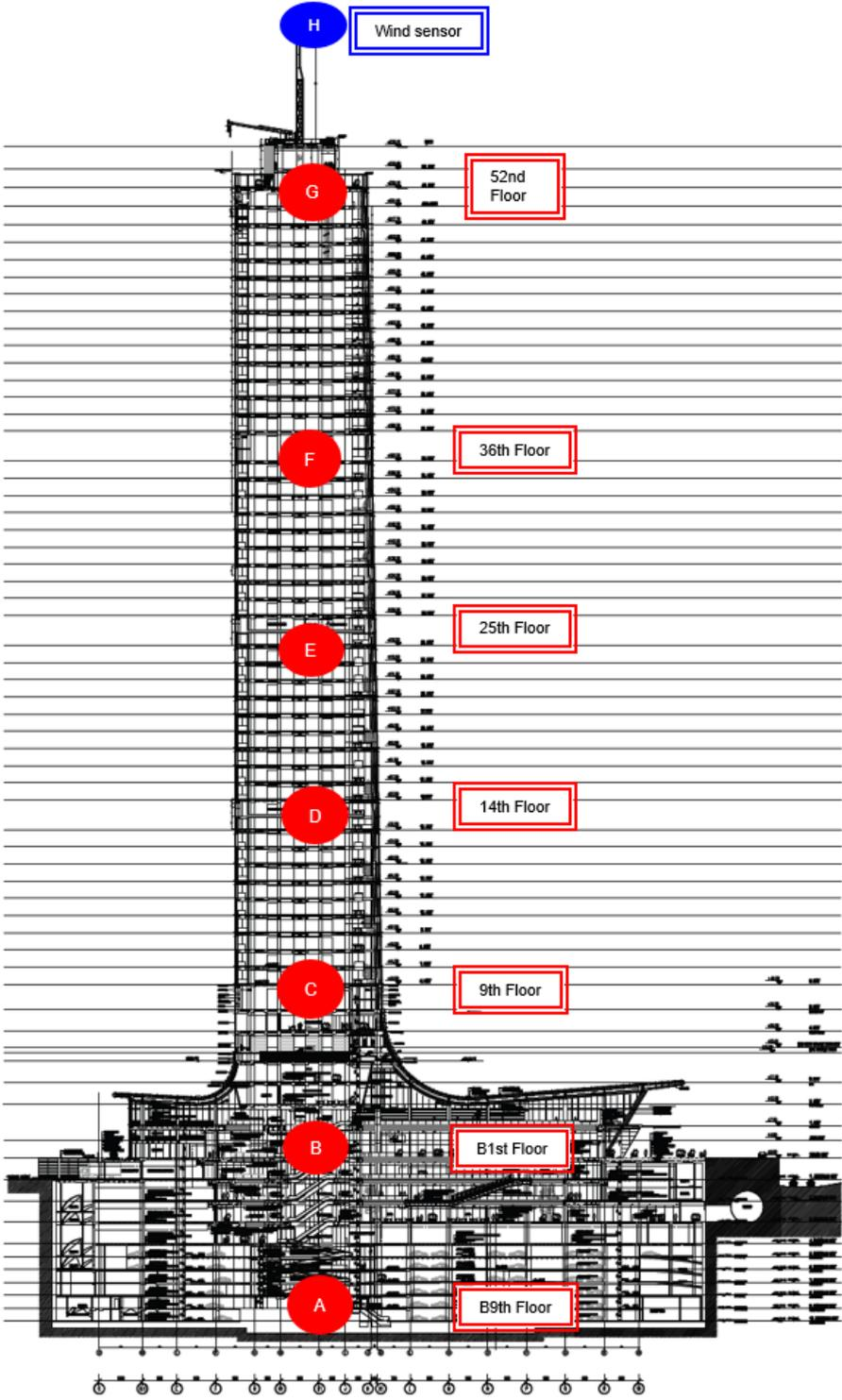
*Fig. I.3. Locations of instrumented floors in the Sapphire building in Istanbul, Turkey.*
