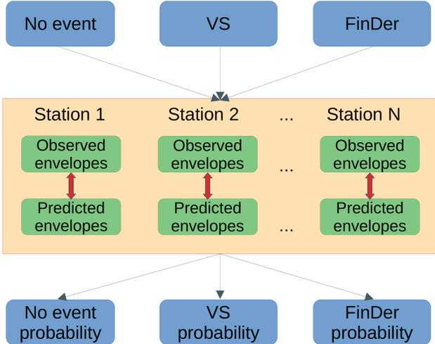
Figure II.7. Overview diagram of the procedure to compare and prefer EEW solutions
