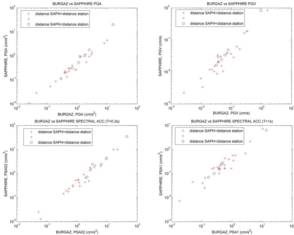
Figure I.6. Attenuation from Burgaz EEW station to Sapphire Bldg. for PGA, PGV, SA(0.2) and SA(1.0)
