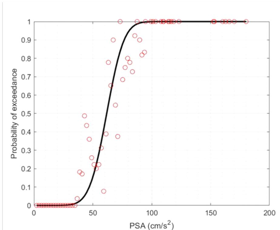
Figure I.10. Probability of exceedance of 2% code drift limit with PSA at the first modal frequency in the E-W direction.
