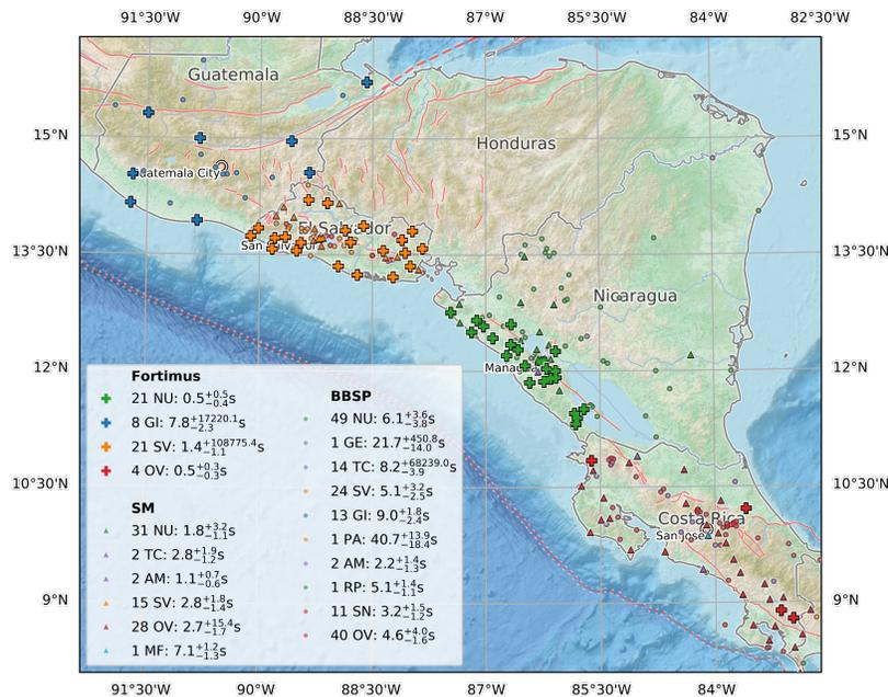
Figure II.4. Permanent seismic network map from October 2022. Stations that include strong-motion sensors (SM) include both force-balance and MEM accelerometers. Stations with only a velocity sensor (BBSP) includes either seismometers or geophones - these will clip in strong motion, though are useful for P-wave arrivals. EEW-ready strong-motion seismic stations (Fortimus) have been deployed from 2021
