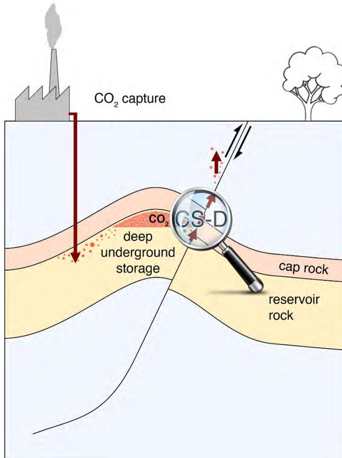
Flow through faults, potential leaks through a cap rock:
